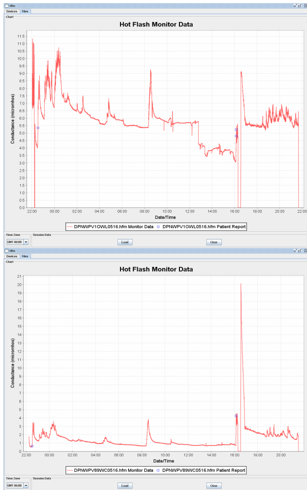
Fig. 3 Side-by-side comparison of two electrodes worn by the same subject at the same time. Top: Biolog cream causes about 6 micromho ( \mu\text{S} ) baseline conductance. Sweating caused by exercise (marked by circles) causes about 30% change. Bottom: Conductive adhesive gel causes about 0.8 \mu\text{S} baseline conductance and has less motion artifact. Sweat caused by exercise causes 400% change. During shower (at about 16:00 hours), the recorder was detached (0 \mu\text{S} ). After shower, electrode was wet, recording about 20 \mu\text{S} and recovering in about 1 h.
